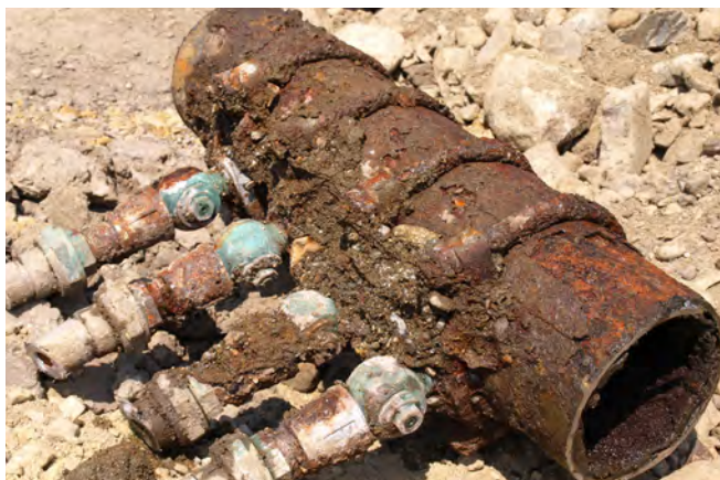
Corroded water main with lead fittings. Photo by Mike Thomas via Flickr, CC BY NC ND 2.0
